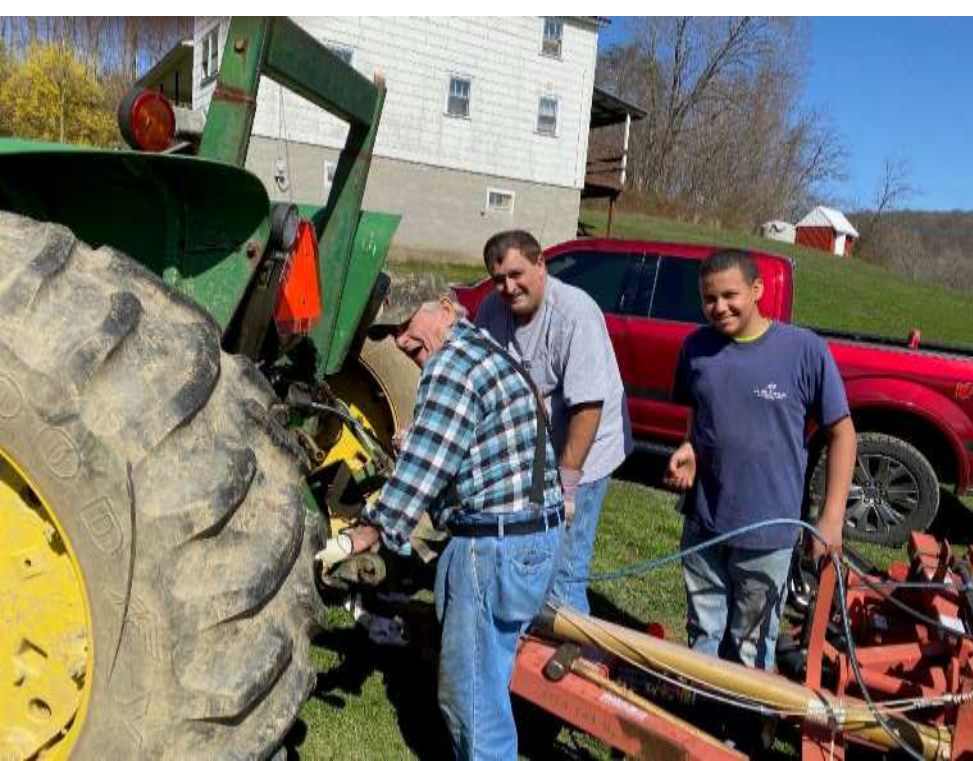
Rodney Shuey, George Pentz, Wyatt Heller prepping the the 15' Batwing finish mower and 8' mower. Blades sharpened, greased, oil checked and tested out. The batwing seems to work well. Hydraulics fold it up nicely.
