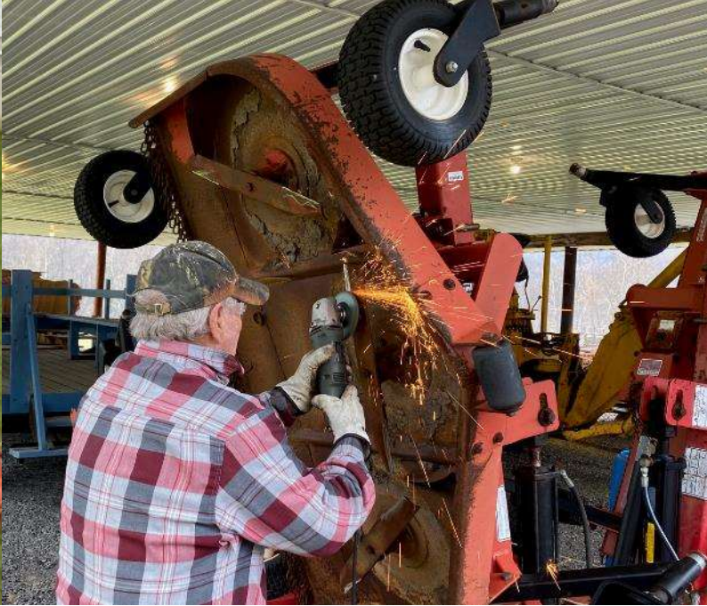
Rodney Shuey, George Pentz, Wyatt Heller prepping the the 15' Batwing finish mower and 8' mower. Blades sharpened, greased, oil checked and tested out. The batwing seems to work well. Hydraulics fold it up nicely.
